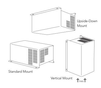
This versatile deck mount converter can be installed in any position, making RV design more flexible for manufacturers.
