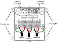
ATTENTION Insert wire properly. Approved torque range 25to35in-lbs. Over torquing will cause terminal damage.
