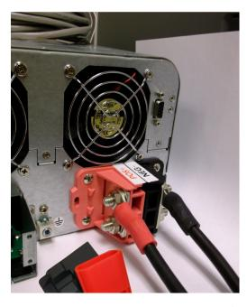
The WF-5118/WF-5120 inverters require 2/0 AWG input cables and a 250 Amp in-line fuse.
