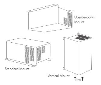
This versatile deck mount converter can be installed in any position, making RV design more flexible for manufacturers. Mount converter vertically with fan at the bottom to enhance cooling. Easy horizontal installation. WF-9800 Series converter can even be installed upside down. BATTERY
