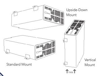
WFCO recommends horizontal mounting of the WF-68100AD series. You can mount it in any position that provides unobstructed ventilation for the fan and vent holes.
