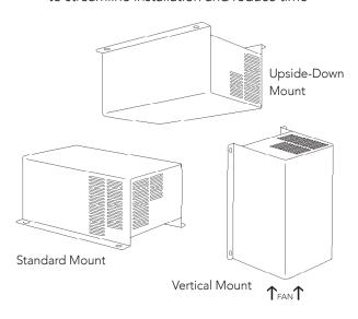
This versatile deck mount converter can be installed in any position, making RV design more flexible for manufacturers. Mount the converter vertically with the fan at the bottom to enhance cooling. WF-8800 Series converter features easy horizontal installation and can install upside down.
