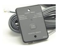
The WF-5110 Series remote includes an ON/OFF button and a 20-ft cable. The switch on the face of the inverter must be in the "out" position for the remote to work.
