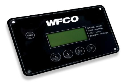
The WF-5220 Inverter remote includes an LCD display and a 32-ft cable. Display includes On/Off button, Battery Voltage status, Grid Input Voltage and amperage status and settings for Battery Under (UVP) and Over (OVP) Voltage Protection.
