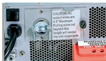
Circuit Breaker to protect outlet from shore power shorts and overloads.
