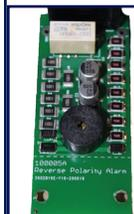
Optional Reverse Polarity Detection meets new RVIA and NEC requirements with audible alarm notification. No additional wiring or hookup is required, and it accepts hi-pot testing.
