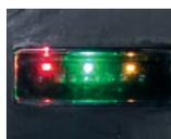
Three AC LEDs inside the door indicate the status of incoming voltage. **Green** is normal. **Yellow** is low. **Red** is too high.
